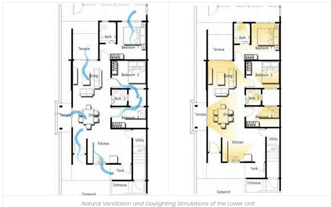
Natural Ventilation and Daylighting Simulations of the Lower Unit
