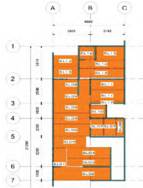
Intermediate Unit Precast Slab Layout
