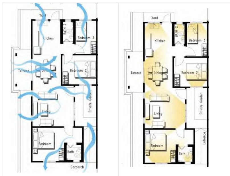
Natural Ventilation and Daylighting Simulations of the Terrace House Unit
