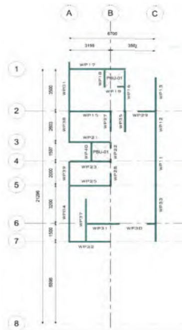
End Unit Precast Wall Level 2 Layout
