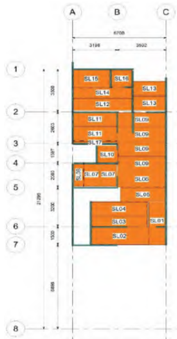
End Unit Precast Slab Layout
