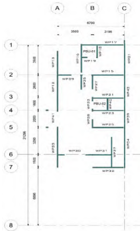
Corner Unit Precast Wall Level 2 Layout
