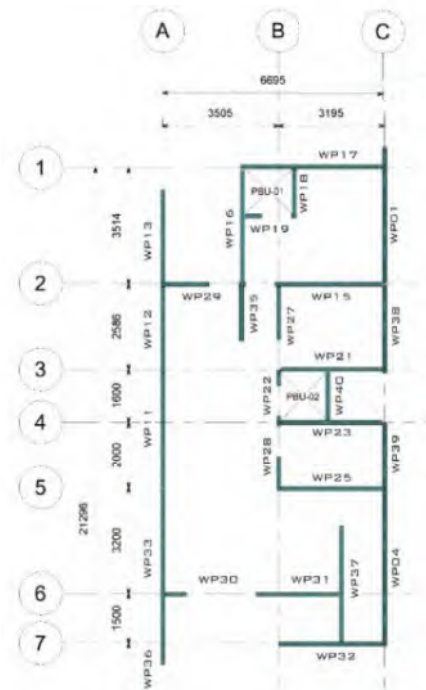
Intermediate Unit Precast Wall Level 2 Layout
