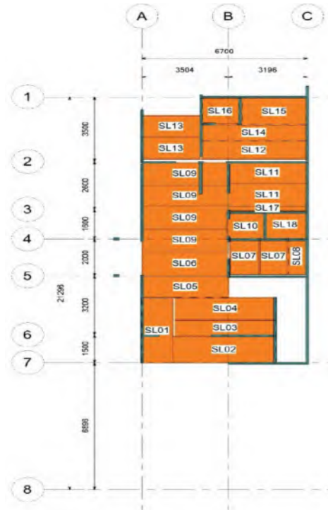
Corner Unit Precast Slab Layout
