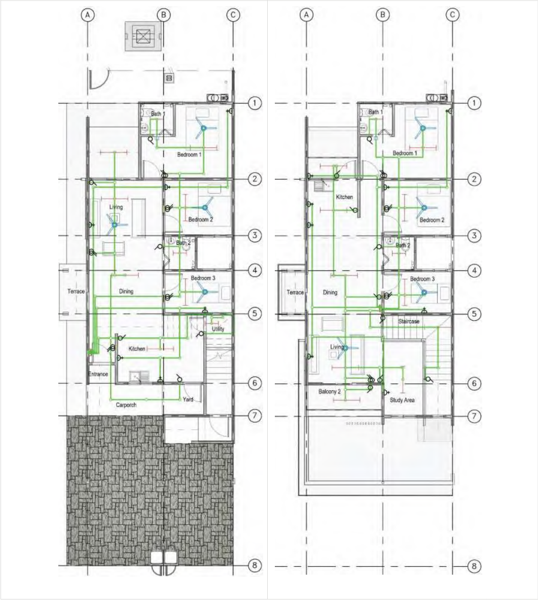
Lighting and Power Layout for the Ground Floor and the 1st Floor
