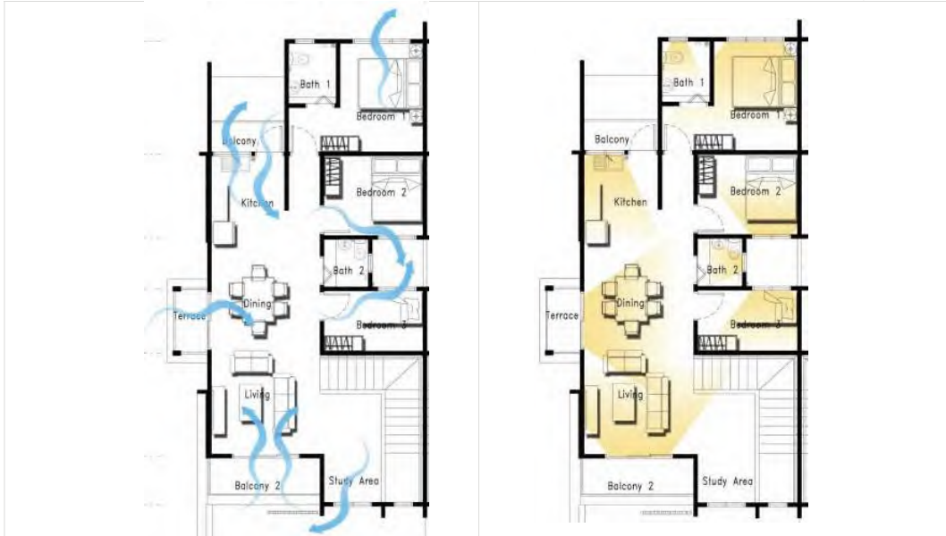
Natural Ventilation and Daylighting Simulation of the Upper Unit
